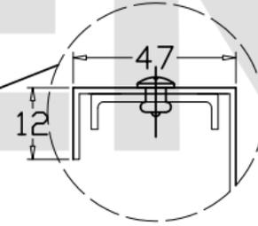
U-shaped stiffeners for connecting cover with drawing nails (5\*39\*5)
